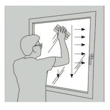
Place squeege or straight-edge alongside window silicon joint, and, using a cutter with a new blade, carefully cut to remove
